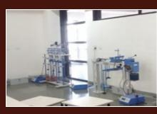
The Geotechnical Engineering Laboratory of Civil Engineering Department, GIDC Degree Engineering College, Navsari houses several instruments and apparatus used by Under Graduate students for their academic purposes. The facilities include testing of soil sample for particle size analysis, compaction, shear strength, consolidation, swelling, permeability, etc. The major instruments are equipped with digital read out unit.
